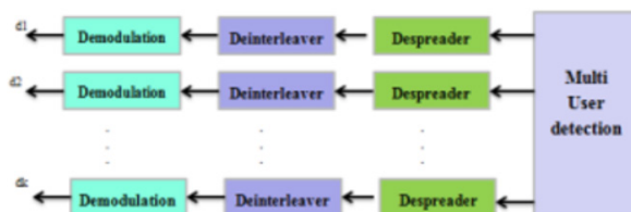
Figure 3. IDMA Receiver block diagram
