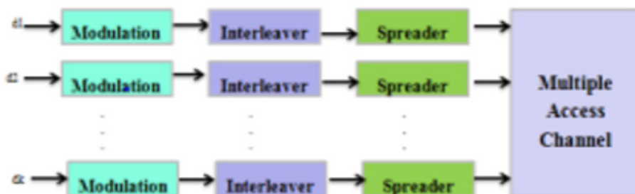
Figure 1. The transmitter structure of an IDMA system with multiple user
